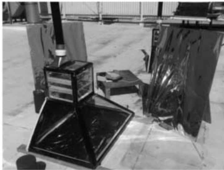
Fig. 1. Solar dryer and two concentrating solar reflection panels used in drying experiments. The data logging instrumentation for the sensors is located on the low table.
